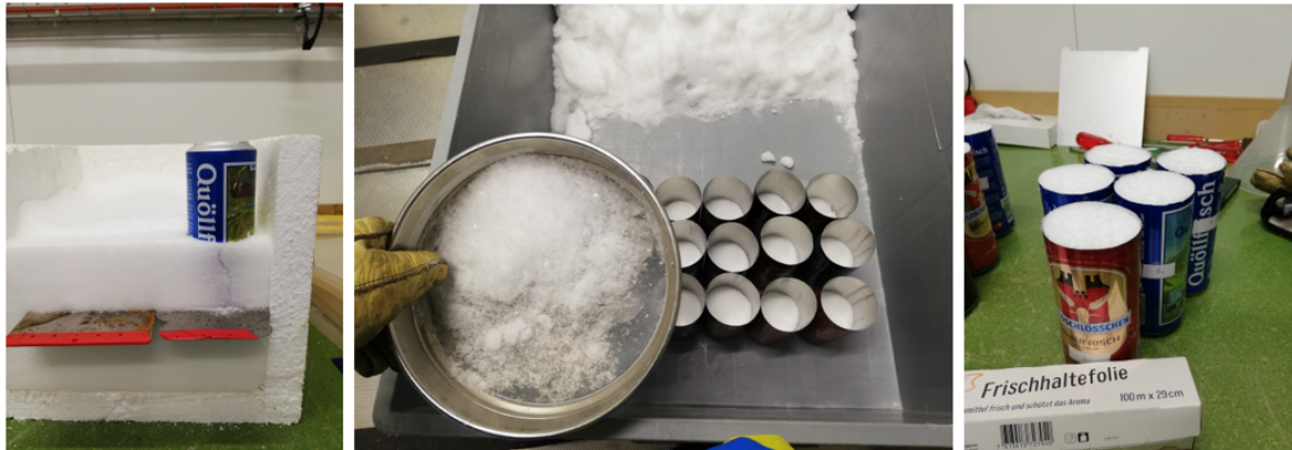
Figure 9: Filling of the cans. Left: filling of the sinthered layer. Middle: filling of the fresh snow layer. Right: filled cans, ready to seal.
