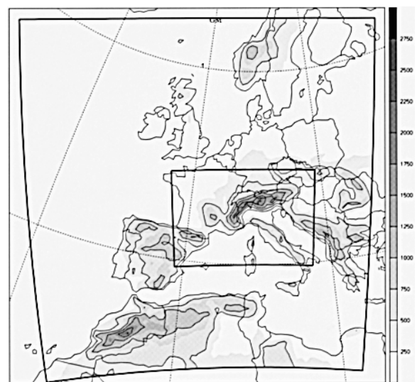
FIG. 2. Horizontal domains for the low-resolution EM simulations (outer frame) and high-resolution HM simulations (inner frame). Shading shows EM topography with additional contours every 500 m.
